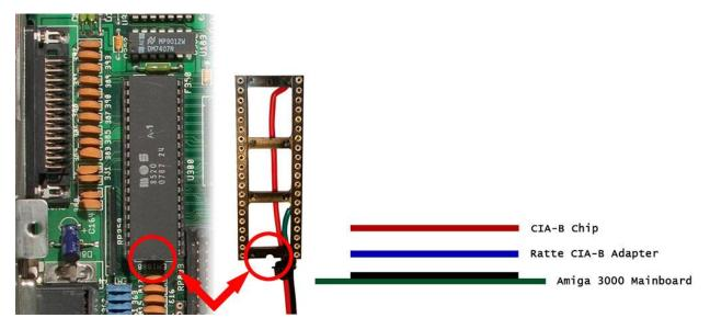
Connect the CIA-B adapter to the Ratte Automatic Monitor Switch as the picture below shows.
