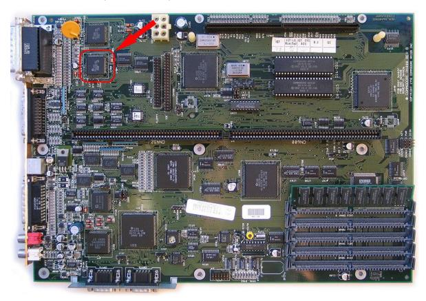
Notice that the corner of the CIA-B adapter is beveled, also is the CIA-B chip (**U300**). You need to align the corners and then gently but firmly push down the connector on top of the CIA-B chip.
