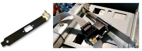
If you have such bracket at home, it is easy to assemble the switch on it. A PCI bracket with a 9 pin serial D-Sub also works.
