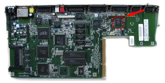
Notice that the corner of the CIA-B adapter is beveled, also is the CIA-B chip (**U8**). You need to align the corners and then gently but firmly push down the connector on top of the CIA-B chip.
