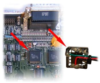
Connect the CIA-B adapter to the Ratte Automatic Monitor Switch as the picture below shows.
