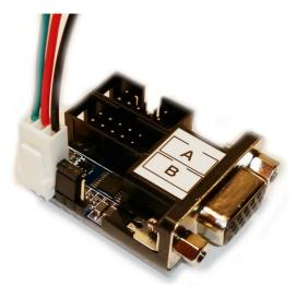
Connect "**A**" to the Indivision / Other scandoubler and "**B**" to the RTG / Voodoo card with the cables that was included in the shipping.
