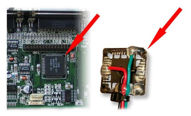
Connect the CIA-B adapter to the Ratte Automatic Monitor Switch as the picture below shows.
